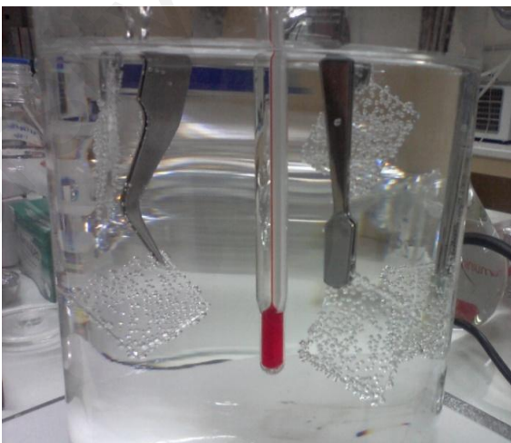
Figure 3.8: Five PMMA sheets immersed in stirring NaOH with temperature controlled at 55°C for 30 min.
