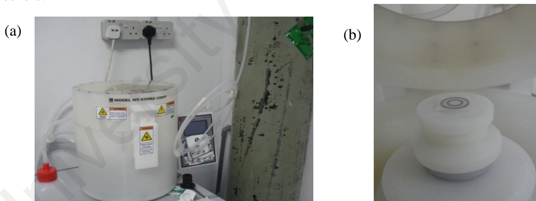
Figure 3.3: a) Spin coater with nitrogen gas cylinder, b) Glass wafer hold onto the chuck by vacuum
